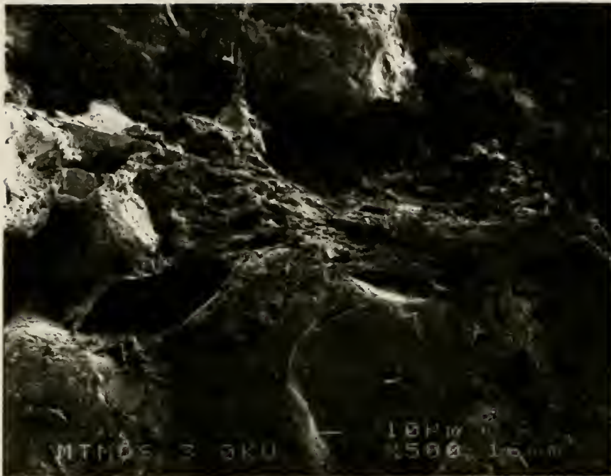
Figure 2.8 SEM photomicrograph of facsimile treated with an ethyl methacrylate/methyl acrylate copolymer (MMA) only and etched with 1M HCl. 3.0KV, 500X magnification.
